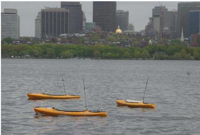
Fig 2: Three MIT “kayak” USVs operating in a network (courtesy Mike Benjamin, MIT)
