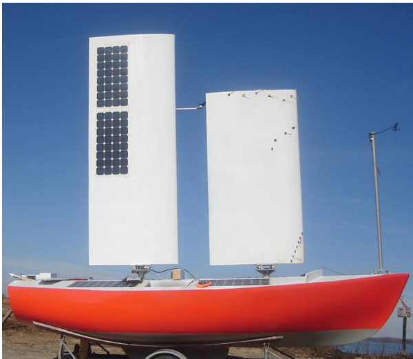
Fig 6: A prototype sailing USV (courtesy Unmanned Ocean Vehicles, Inc.)
